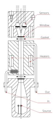
controlling the energy that reaches the detector. This design can be expanded up to 3 gas variables.
