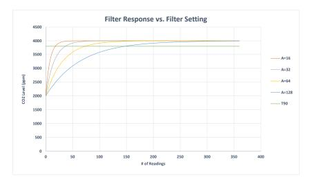
The graph above shows the effect of the filter on response times. Increasing the filter setting increases the measurement output response time.  $T_{90}$  is the time to 90% of reading. The SprintIR®-R takes 50 readings per second. The flow rate was set at 0.2I/min.
