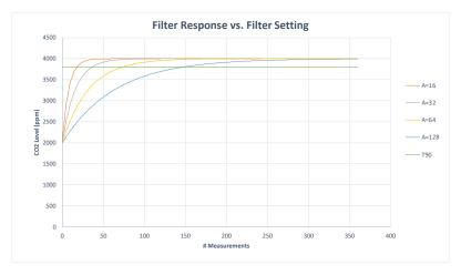
The graph above shows the effect of the filter on response times. Increasing the filter setting increases the measurement output response time.  $T_{90}$  is the time to 90% of reading. The ExplorIR®-M takes 2 readings per second.
