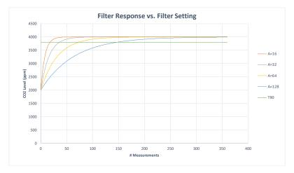
The graph above shows the effect of the filter on response times. Increasing the filter setting increases the measurement output response time.  $T_{90}$  is the time to 90% of reading. The CozIR®-A takes 2 readings per second.
