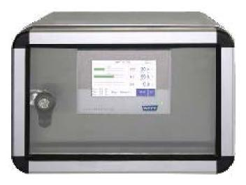
Gas mixing systems for 2 or 3 defined gases, designed for packaging using a protective atmosphere in the food industry. The KM-FLOW uses electronic mass flow controllers (MFC) instead of conventional proportional valves for mixing gases.
