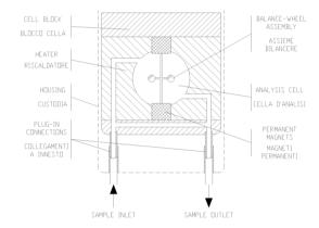
When the surrounding gas contains Oxygen the spheres are pushed out of the magnetic field caused by the relatively strong Para magnetism of Oxygen. The force on the dumb-bell is corrected by a current through the coil which is controlled by a photo-detection system via a light beam and the mirror on the dumb-bell.
