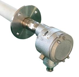
The 6801 Zirconia probe is a resilient in situ analyser, completely ceramic-made, designed for continuous O2 measurement in flue gas at high temperature. The extremely simple and functional design is the result of a long applicative experience
